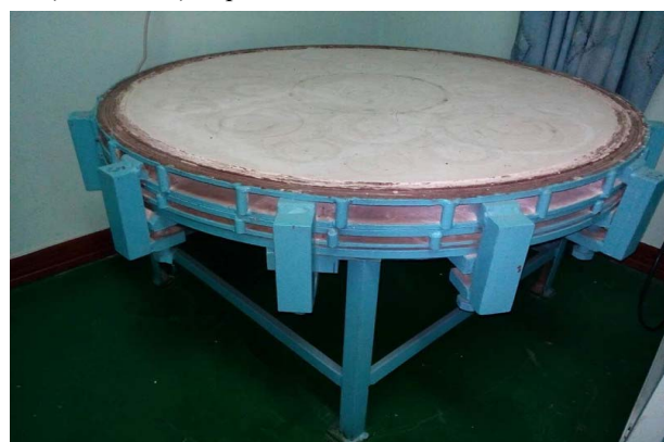
图5 氡析出率测量仪检定装置图 Fig.5 Radon exhalation rate meter verification device image.
